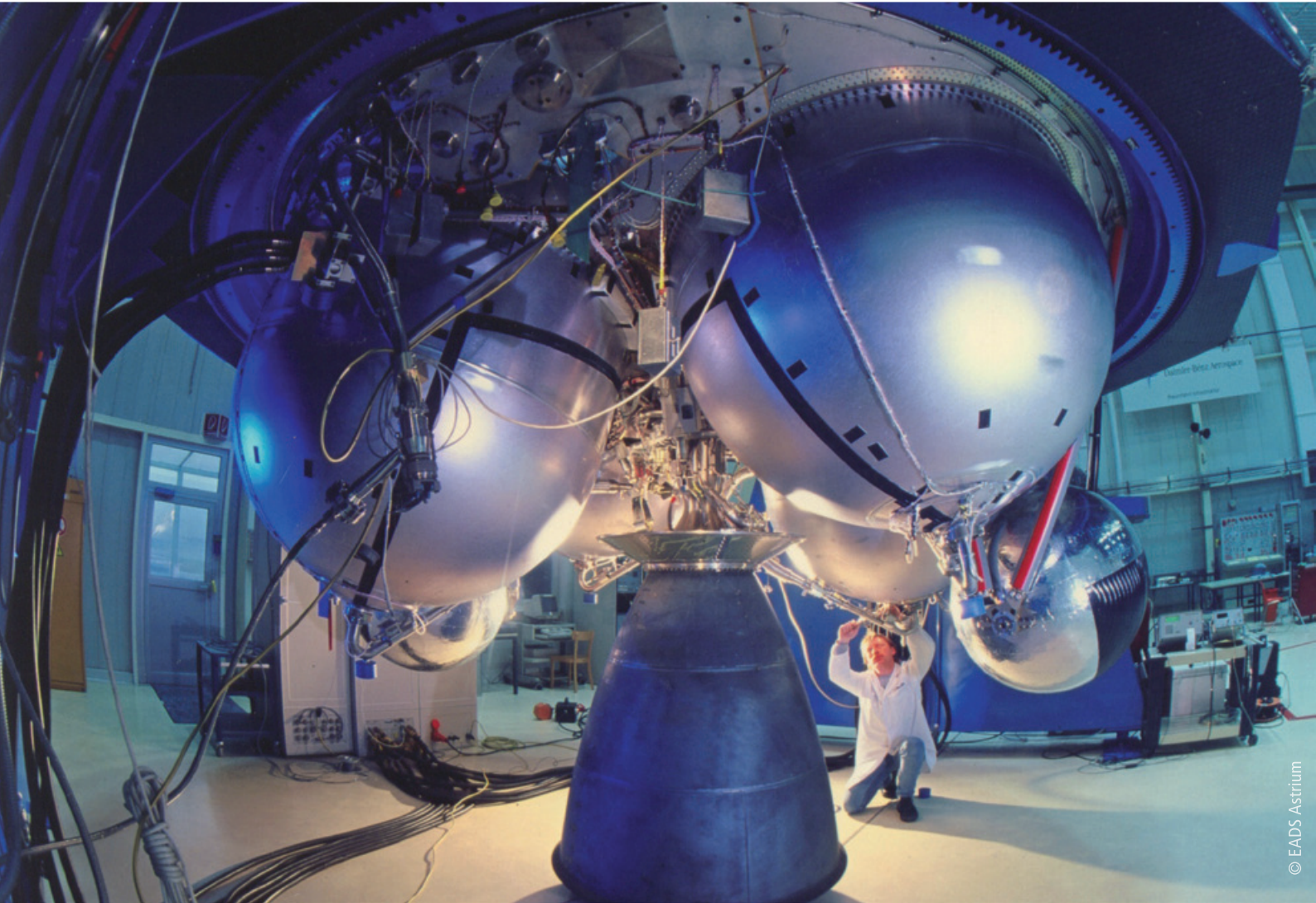
Ariane 5 EPS upper stage with BUTTING piping systems and feed lines
