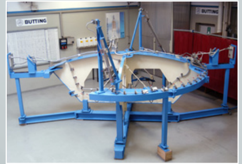
Welding and testing equipment for the EPS upper stage of the Ariane 5 to monitor the geometrical position of the prefabricated piping components
